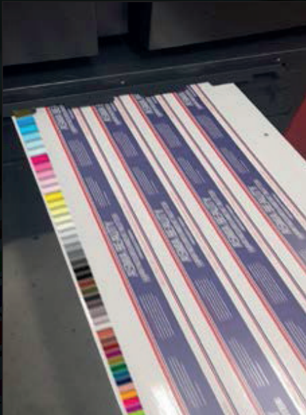
Control strip at the edge of the web
